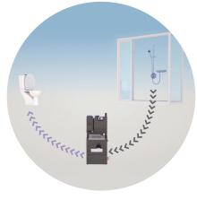
It makes no sense to flush toilets with perfectly good drinking water. Only two showers per day can provide enough water to the Greyter HOME to meet the toilet flushing needs of a family of four.
